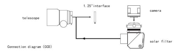
To connect the SLR camera, unscrew the 1.25' adapter under the eyepiece holder, mount the adapter ring (M54-F to M48-M) and then connect the camera bayonet.
